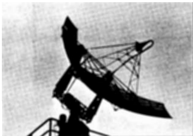
Figure 5. U.S. Air Force FPS-6 height finding radar: 5 MW peak power; 3.5 kW average power.
